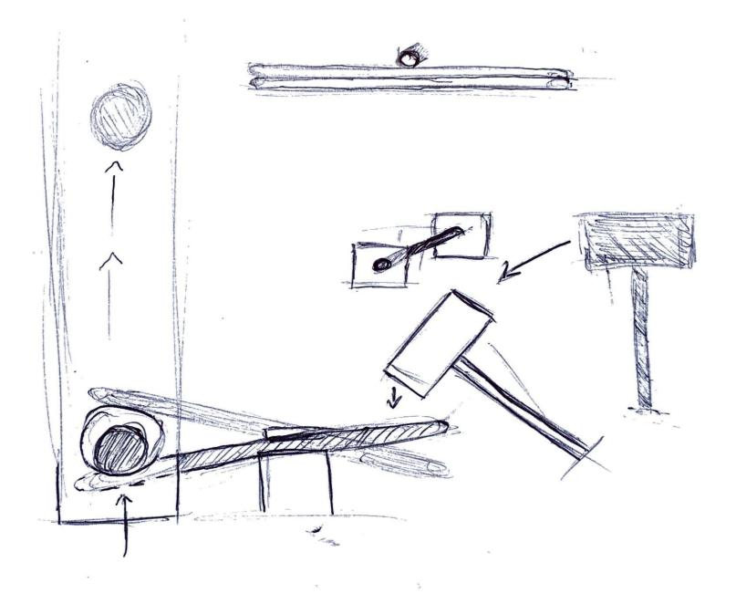
Concepts being brought together. Once the ball is blasted by the seesaw the ball will be able to reach its next destination. A simple cut out will allow the ball to meet its next mechanism which would open a path for the magnets potentially meet. With a simple push of the magnet the next object would fall to meet the mouse trap as the final step.
